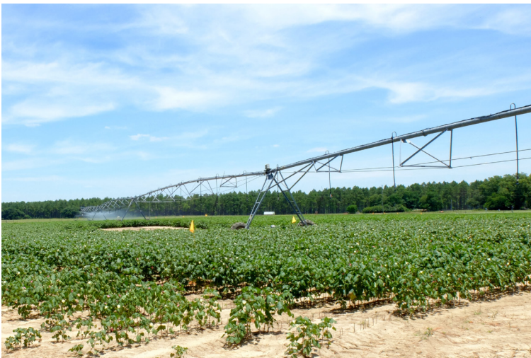
A variable-rate irrigation system being tested at Stripling Irrigation Park, Camilla, GA
