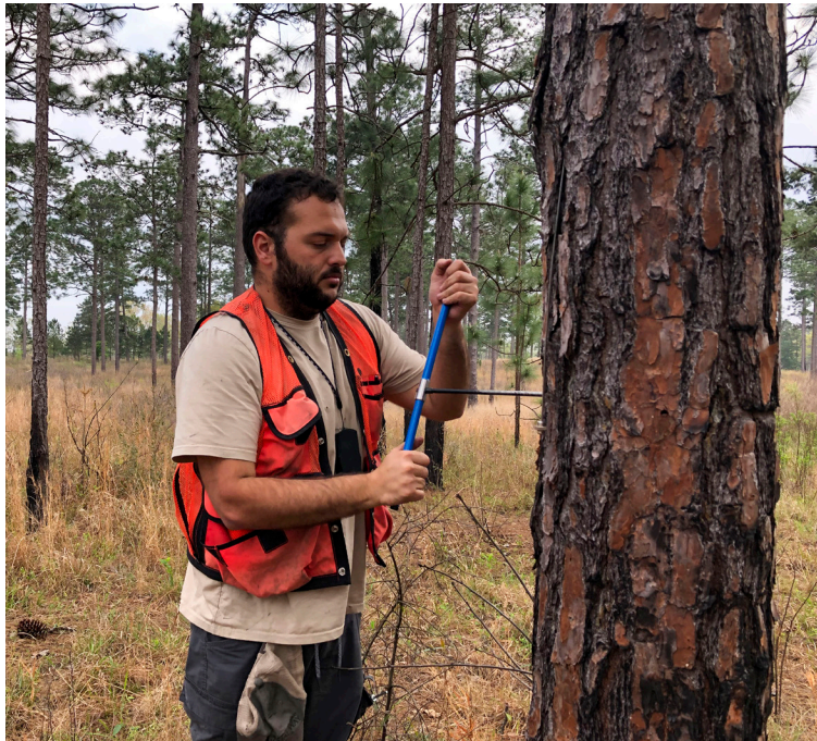
Campôa cores a pine to obtain a tree ring sample for growth analysis. Photo by Joshua Puhlick
