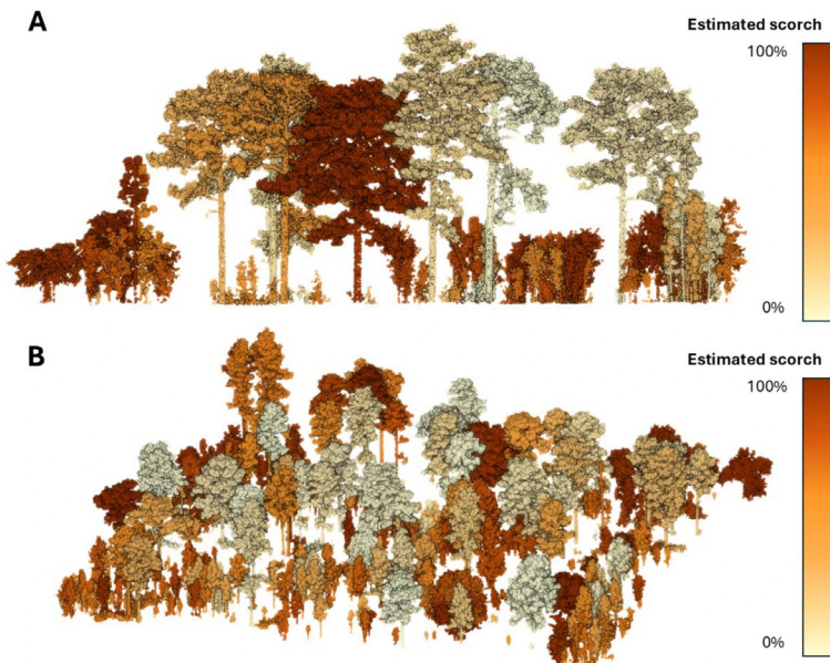
Demonstration of lidar-derived crown scorch prediction for individual trees automatically segmented within (A) a 30 m by 60 m transect and (B) a 1.44-ha portion of the 15-ha study area
